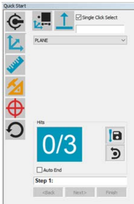
Quick Start showing Plane-Line-Point Alignment
