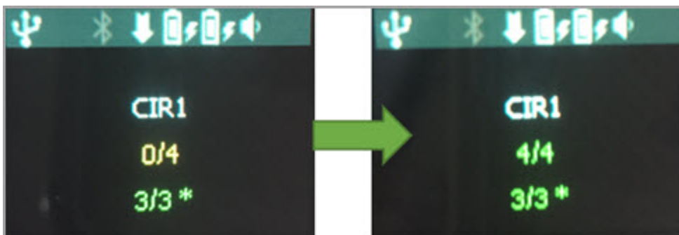
RA8 wrist display for contact auto feature - feature hits
