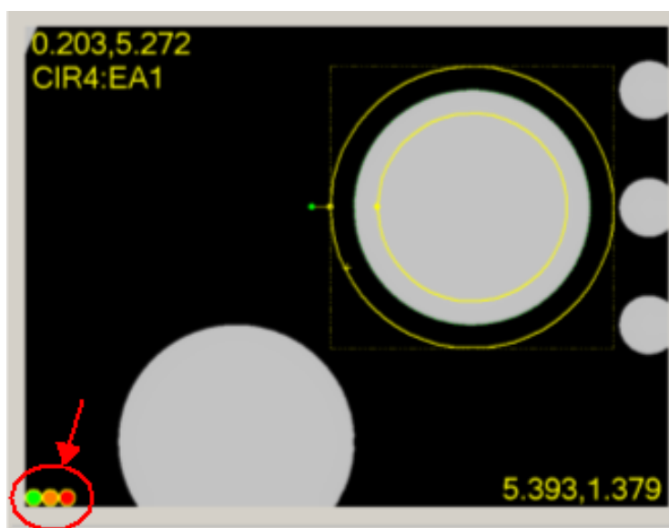
PC-DMIS Vision - Live View showing the colored light countdown
