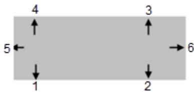
Square Slot measured with six hits
