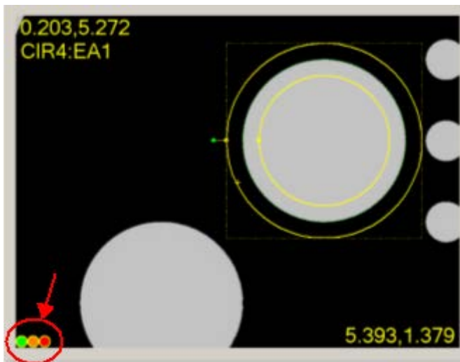
PC-DMIS Vision - Live View showing colored light countdown
