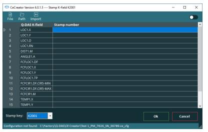
During the installation of the Q-DAS Converter, the CeCreator can also be installed by activating the corresponding checkbox. This tool can be used to change the values of the K-fields **K2001** or **K2002** for the result file.
