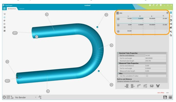
The problem with this method was that tube benders consider this as two separate bending operations.
